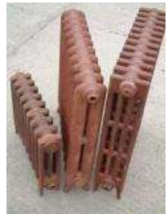
FIGURE 2. Cast iron radiators
